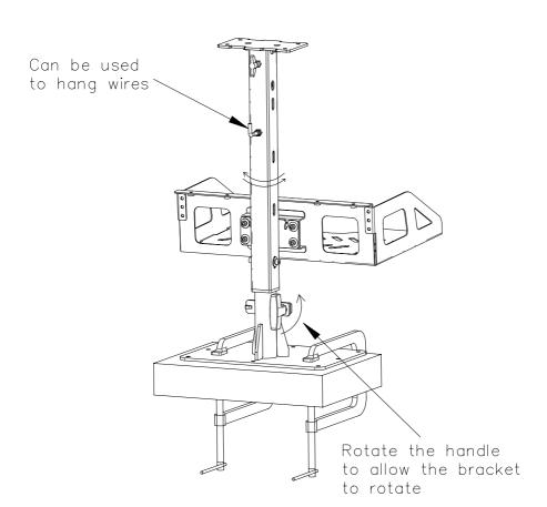
Rotate the handle to allow the bracket to extend and retract and screw it back to fix the height you want
