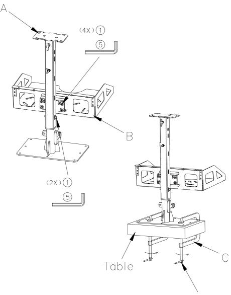
Rotate the G-shaped clamp to secure the bracket to the table
