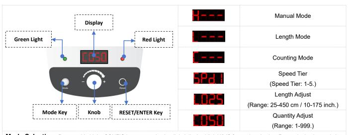
**Mode Selection:** Press and hold the CONFIG button to make the digital display blink H/L/C for mode selection. Rotate the knob to switch between modes, and press ENTER to confirm the current mode
