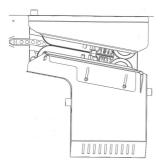
Remove the upper and lower cover by removing the 3 screws (1 screw on the upper cover and 2 on the lower cover)
