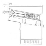
a. Install the upper and lower cover by tightening the 3 screws.(1 screw on the upper cover and 2 on the lower cover)
