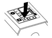
When the machine is in a stop state, press the loading button to enter the film-loading mode, at this time the upper and lower belts will pull the air cushion film slowly forward to a certain distance and then stop automatically.
