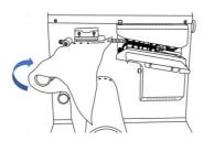
And then sleeve the air cushion film opening to the nozzle, drag the film toward the arrow direction to reach the gap between upper and lower heating belts.
