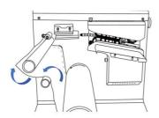
Place the air cushion film on the mandrel, with the inflatable end close to the machine, lead the film through the middle of the 2 guide film rods.
