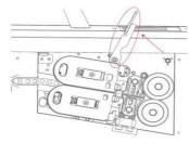
Rotate the lifting handle counterclockwise until the handle is turned to the far left position, so that the two rubber wheels are separated from each other and the upper cooling block rises automatically
