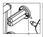
a. Place the air cushion film on the mandrel, with the inflatable end close to the machine, lead the film through the middle of the 2 guide film rods(2), and then sleeve the air cushion film opening to the nozzle(3), drag the film toward the arrow direction to reach the gap between upper and lower heating belts
