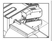
b. When the machine is in a stop state, press the "Trans-film" button enter the film-loading mode, at this time the upper and lower belts will pull the air cushion film slowly forward to a certain distance and then stop automatically.
